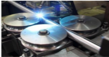
TIG Welding Pipe
